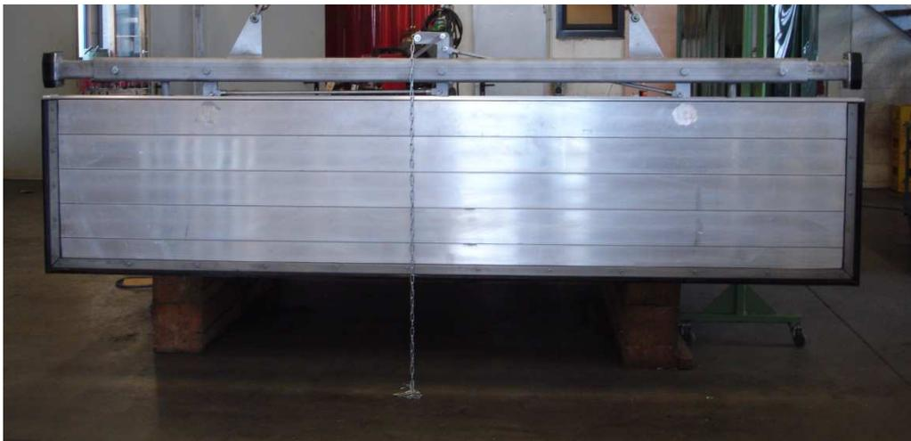
Fig. 07 (Lifting beam with stop log)
