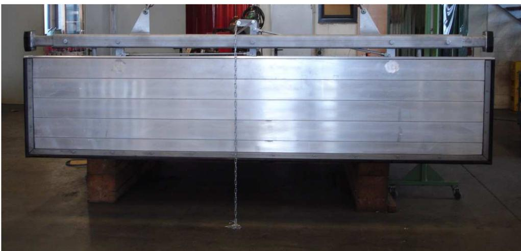
Fig. 04 (Lifting beam with stop log)
