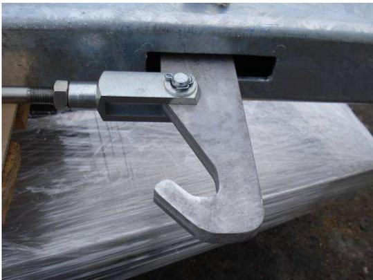
Fig. 02 (Lifting hook)
